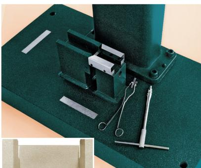
The specimen rests horizontally on the Charpy supports. Centering tongs can be seen in front.
