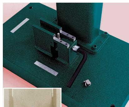
The specimen is clamped vertically at one end, using the front screw/vise. Left: The striker.
