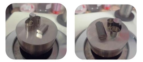
After cutting operation small pieces mounted with ECOPRESS 100 mounting machine. Acrylic based powder (NET) used for mounting operation.
