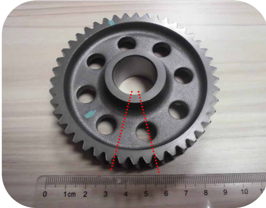
Sample dimensions and requested cutting directions. (Hardness 45~50 HRC)
