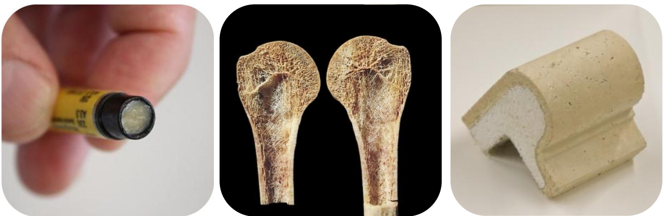
Some examples for cold mounting which can be damaged in hot mounting processes
