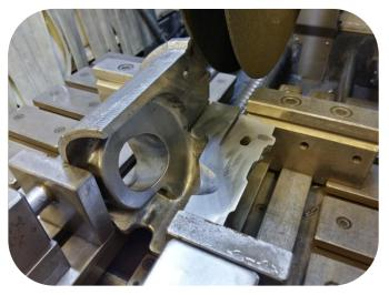
Cutting parameters for small piston : Feedrate:  $100 \ \mu/sn$ RPM:  $2200 \ r/min$ Time:  $21 \ min$
