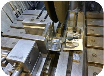
Big one was fixed to the table with GR 0029 and GR 0030 Quick acting clamping vises. Requested width:  $\rm 30mm$
